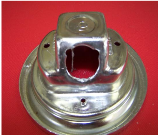
7. This is the starting of filing some material away to make the correct fit.
