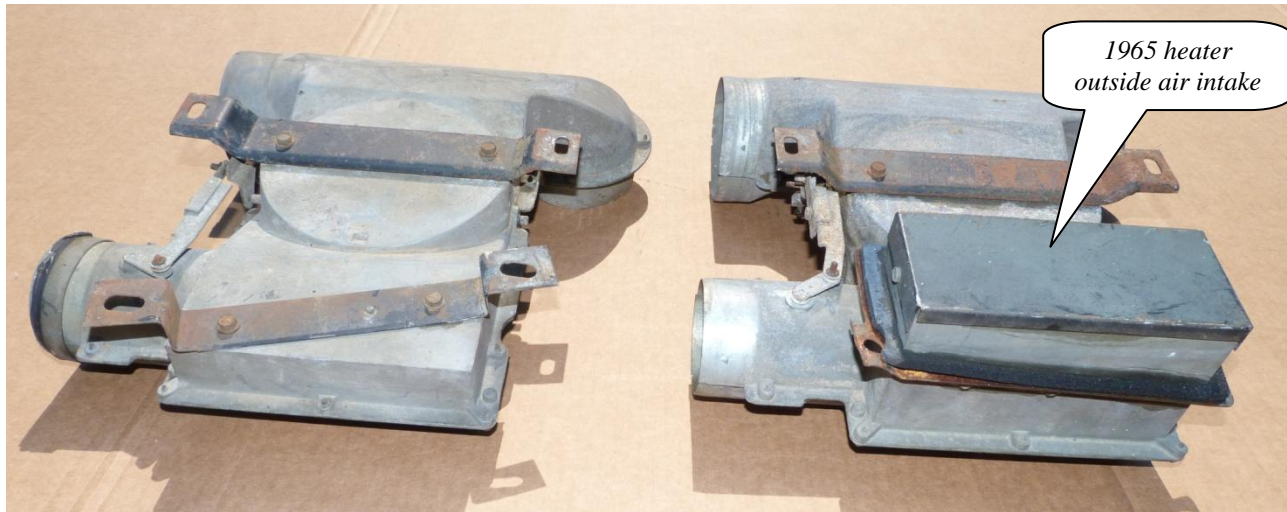
Late model heater boxes. 1966-1969 style on the left, 1965 style with fresh air inlet box on the right.
