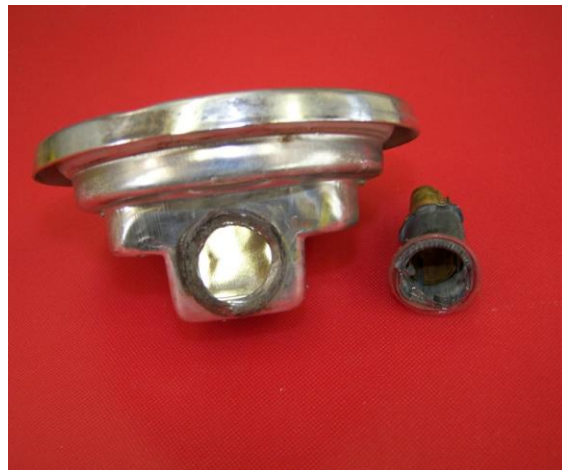
4. I have removed the original socket from the backup light fixture
