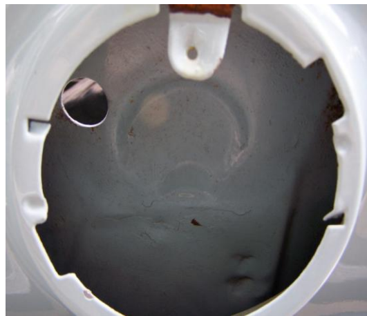
2. Backup light hole showing tabs that you use with blank covers.
