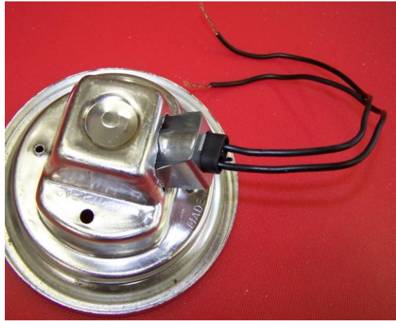
6. You need to file out the round hole so that the square socket will lock in place
