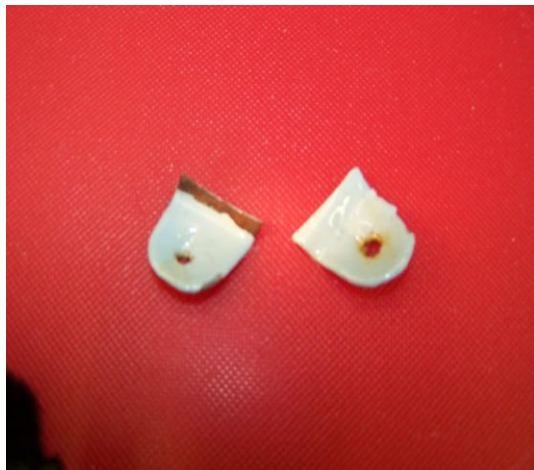
3. This is a shot of the two tabs you bend and break off to install the backup light fixture.
