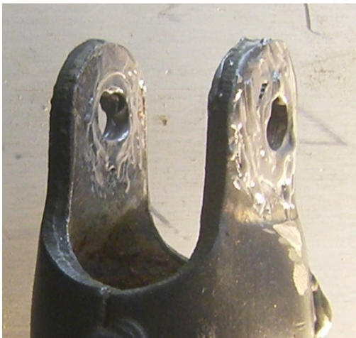
JB weld doughnut into place
