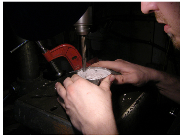
Carve away the unwanted bondo. Not a simple task as you need to leave as much strength material as possible.
