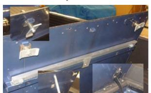
left: Eric Taylor uses hinges that tucks into the heater box cavity (inset). He built a holder for his prop into the bottom side of the panel (inset). and has two turning latches to hold down the lid(inset).
