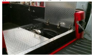
above: Russ Thulen had to raise the cover 4 inches for clearance on his turbo charged Rampside. He used a split diamond plate panel system with cabinet style spring-loaded hinges that hold the panel when opened fully.
