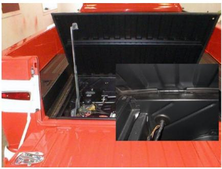
Above: Dennis Dorogi uses recessed hinges (inset) on his for an original appearing floor. He added a standard Corvair car hood support. Being a lefty he wishes he had put the support on the right side for more clearance.
