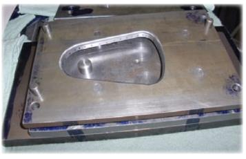
Dann enjoys designing and building the forms, dies and stamping plates. Above and below is the fixture used to punch the hole for the handle
