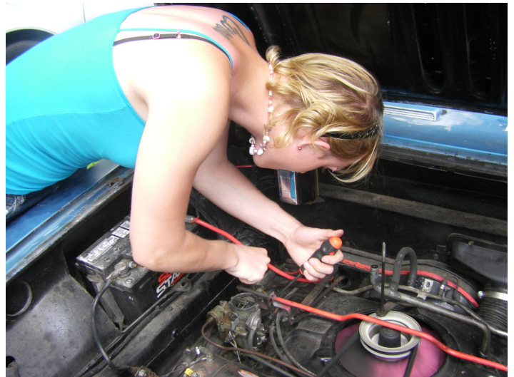
Ashley turns up the idle air screw on her driver's side carburetor since the engine idled a bit slow in Drive.
