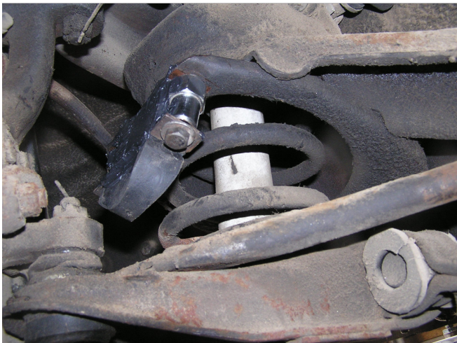
This third photo shows an overall view of the extended Rebound bumper directly above the brake reaction rod on the lower control arm. The Lower Ball joint is to the left and the sway bar's left end is visible on the lower right corner of the picture. This is the 'empty car' position for these parts.
