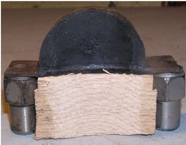
Here's a view of my old "Snubber" with its new curved OAK block to take the hits, along with some steel parts to hold the bolts.
