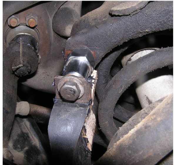
This second photo shows how it looks installed – pointing down – at the lower control arm. See how the curved OAK just clears the spring in its tower.
