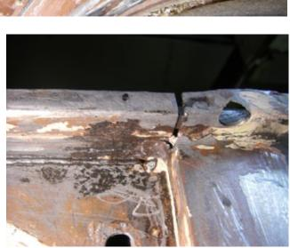
I plan to expose all four clip areas and then Acid etch the rusty stuff; followed by Epoxy and the final paint. I am toying with the idea of a black Rampside with a Silver stripe, roof and wheels.
