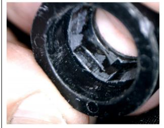
Now I will ZOOM in on one of the flats to show you the pile of scraped up material I made when I forced the assy on to the rubbing block.
