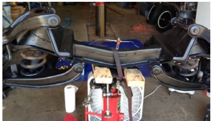
It was much easier to disassemble and clean the crossover and a-arms with the suspension out of the truck.
