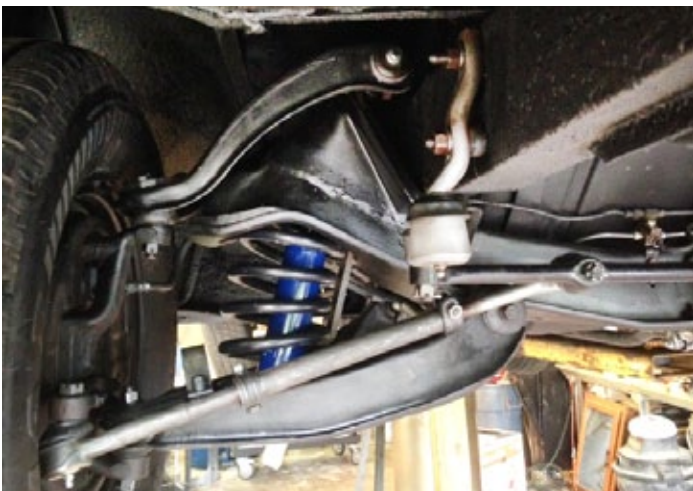
Left: New springs and shocks are installed.
