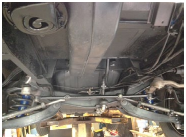
The refurbished suspension is placed back in the truck notice the NOS boomerang (steering relay).
