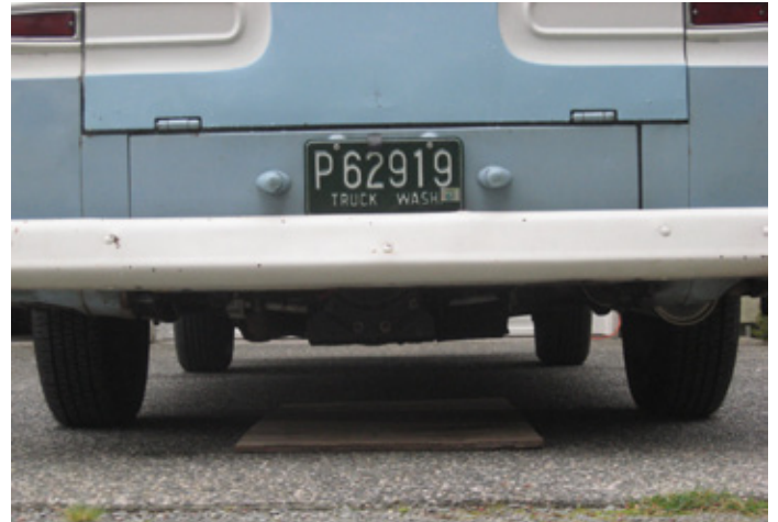
After reinstalling the shortened springs the tires fit flat on the ground. Allowing the more of the footprint to share the load.
