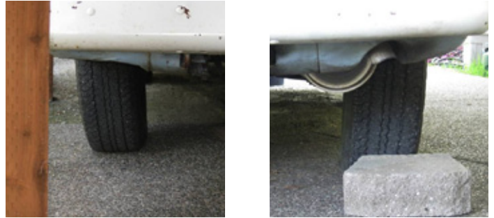
Before the typical FC positive rear camber that eats the outside of the tire.
