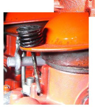
This photo shows how the sharp end of the steel clamp engages the hole in the Carb's Aluminum air horn.
