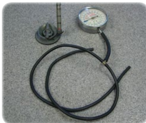
Uni-Syn gauge and vacuum gauge with hoses.
