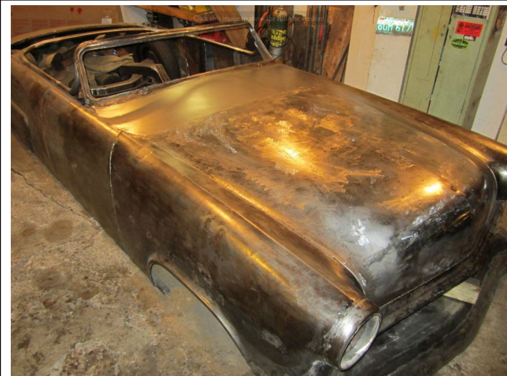
My front fenders and hood are all welded to the body.
