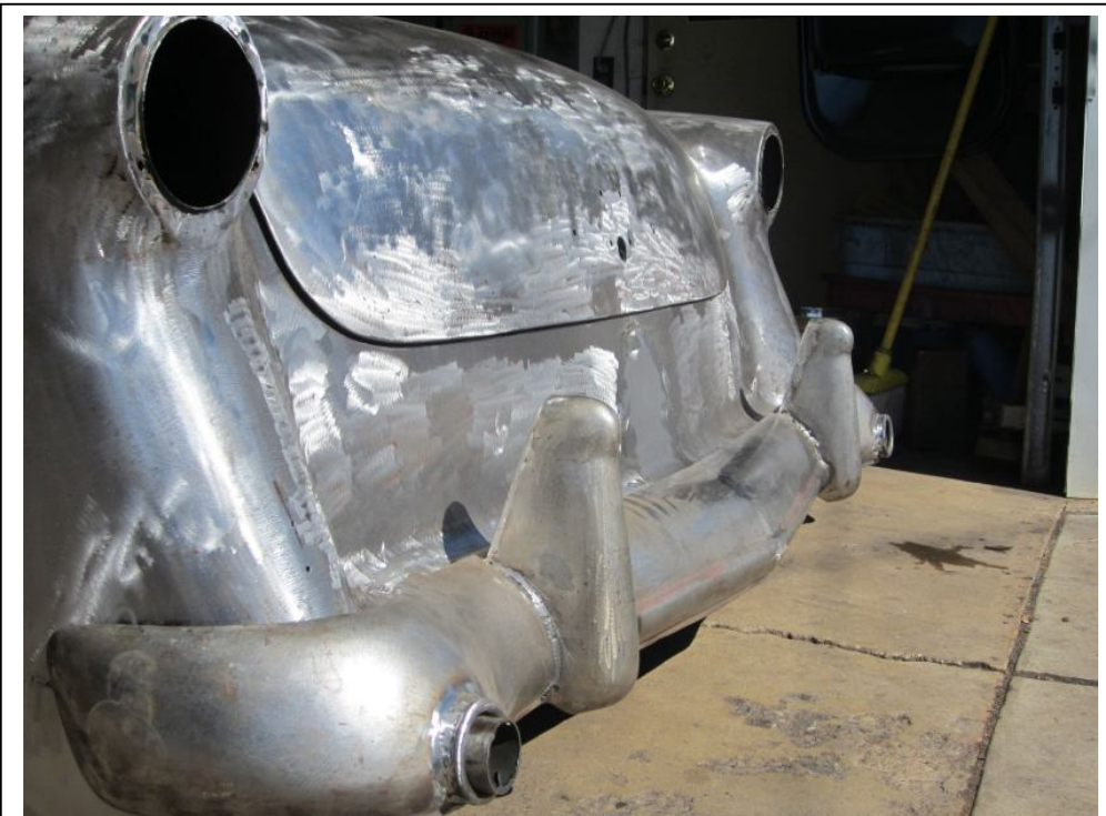
I narrowed the rear bumper a couple inches so it would fit tight up against the body. Then I made holes for the exhaust.
