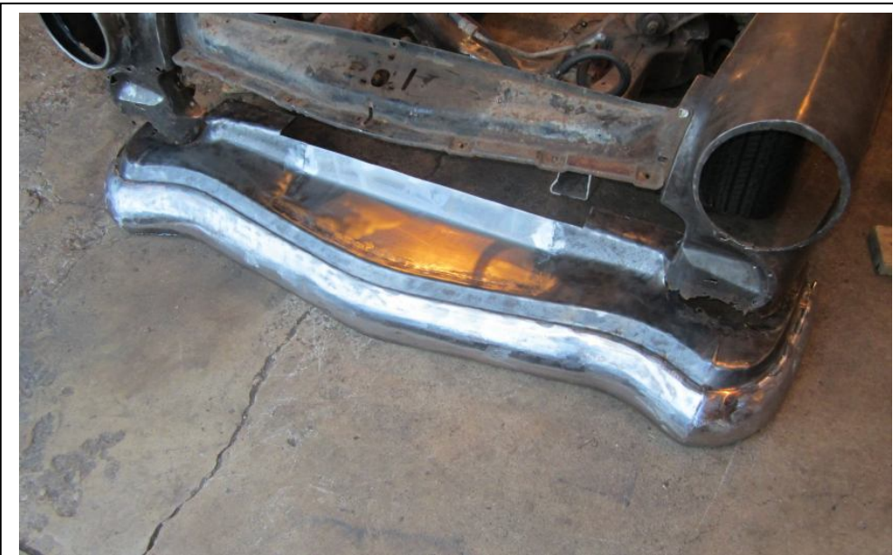
Front bumper and splash pan welded in.
