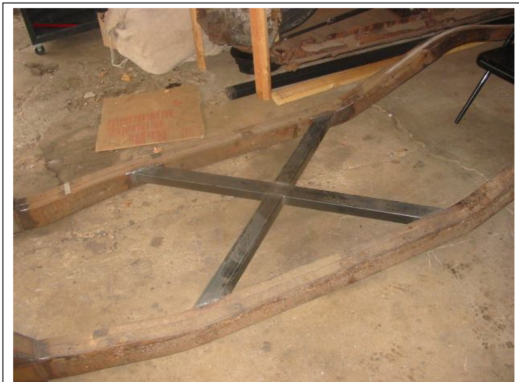
This is March of 2012. I built a very tough x-member for the frame.
