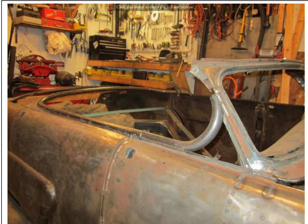
I grafted roll bar tubing along the top of the doors and windshield.
