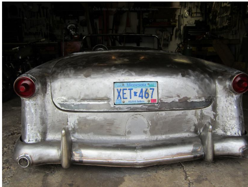
I recessed my licence plate into the trunk lid. It is also the latch for my trunk.
