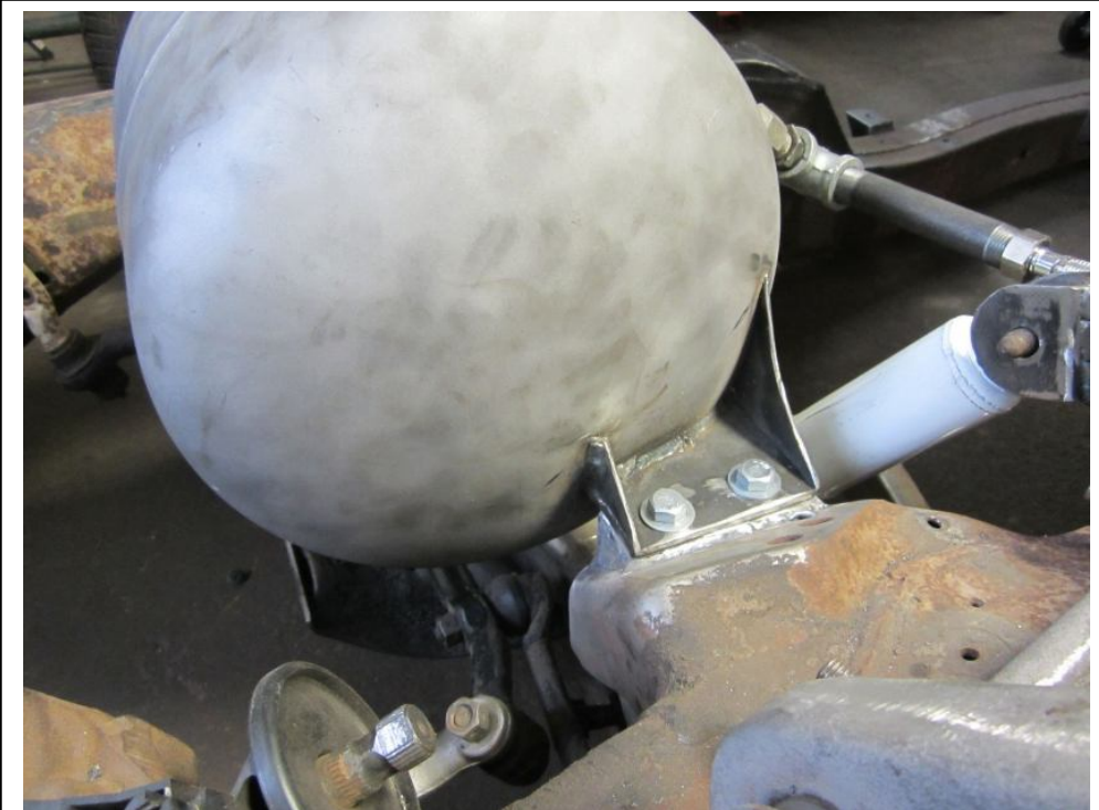
Where there would normally be an engine in the S-10, I mounted a 5 gallon air tank.
