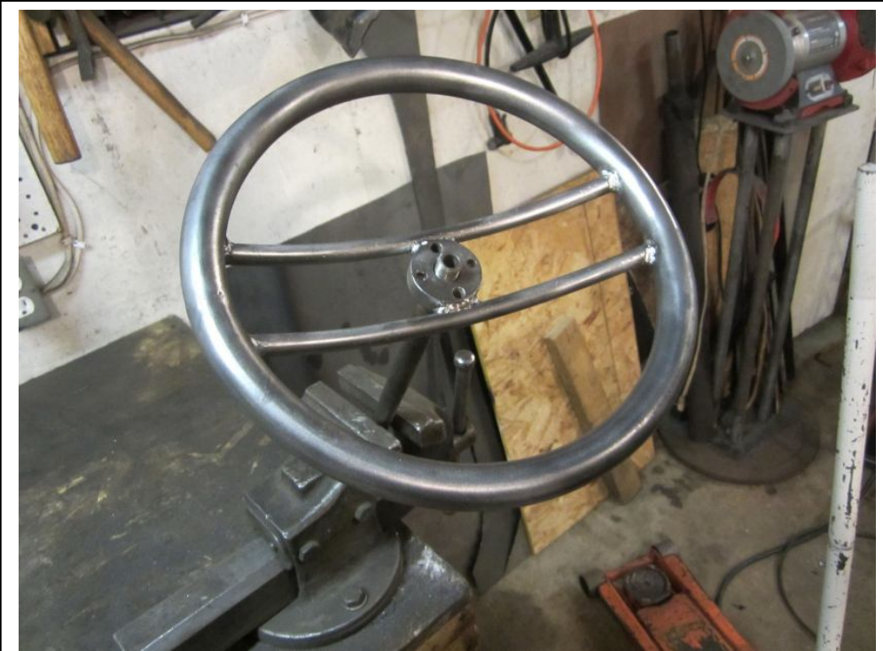
My buddy, Beau helped me make this 10 inch wheel with his Harbor Freight tubing roller.
