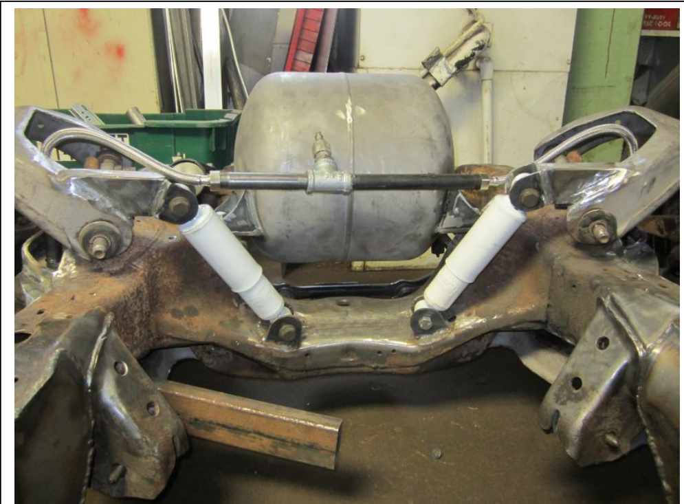
My shocks run backward off of the upper control arms. I looks wrong, but works good.
