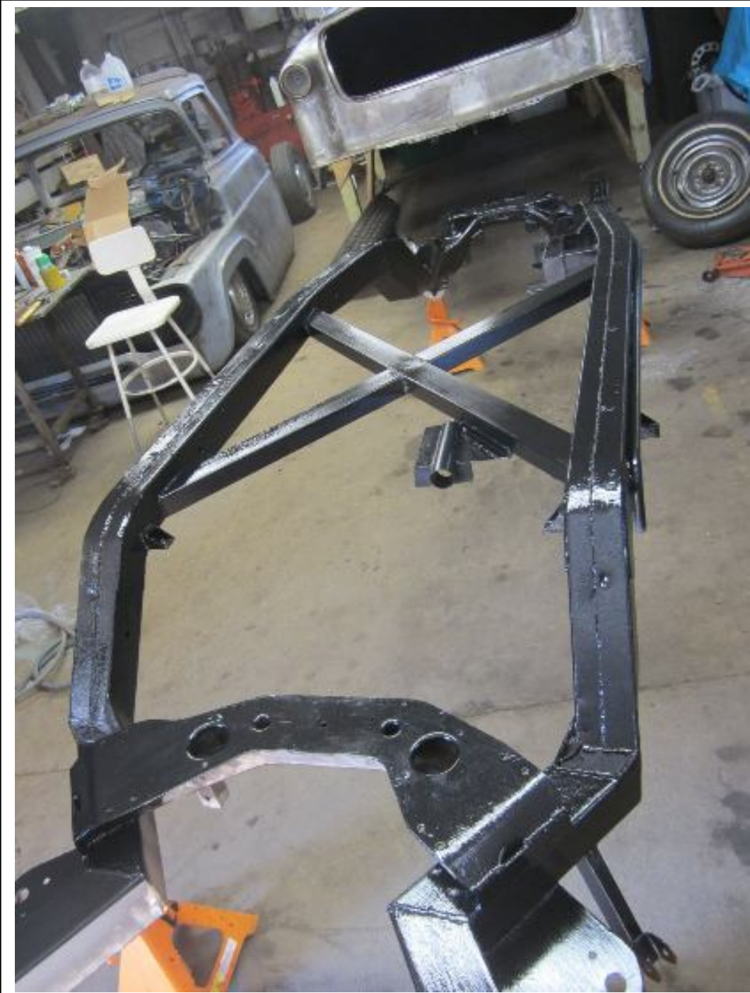
Sandblasted and painted frame.
