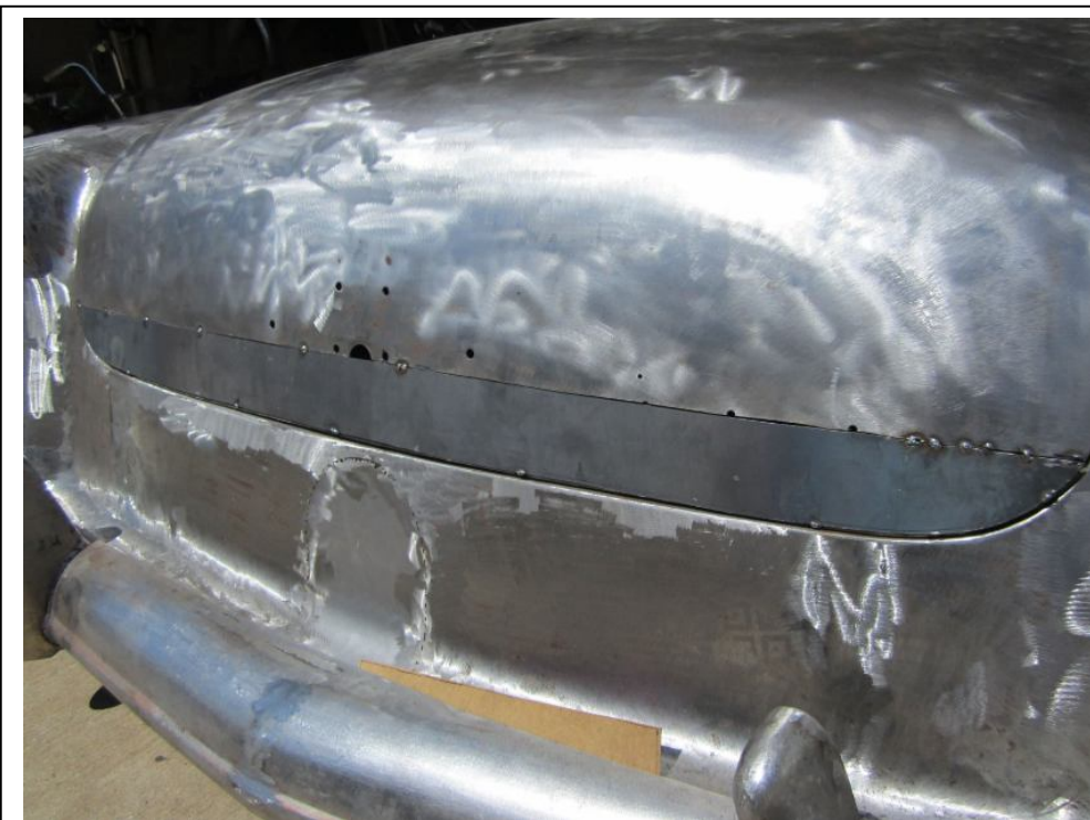
The bottom lip of the trunk lid needed some rust repair.
