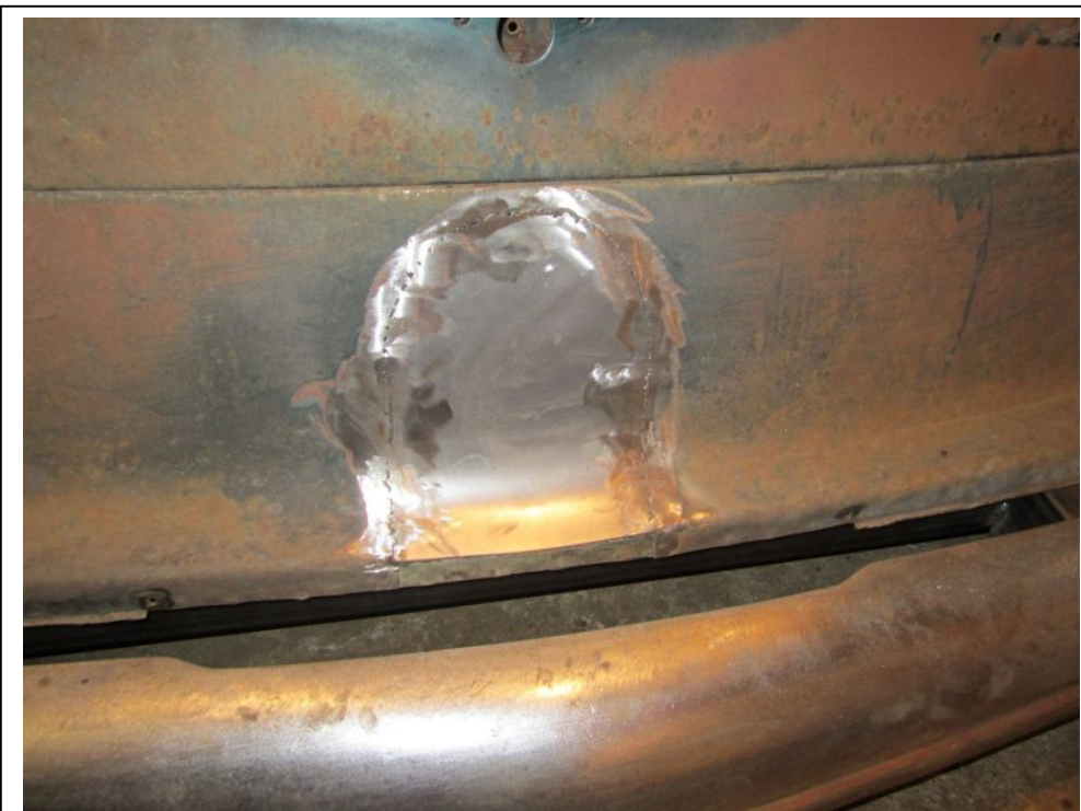
Filled the gas door.
