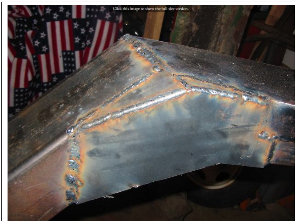
A little 12 gauge to hold it all together.
