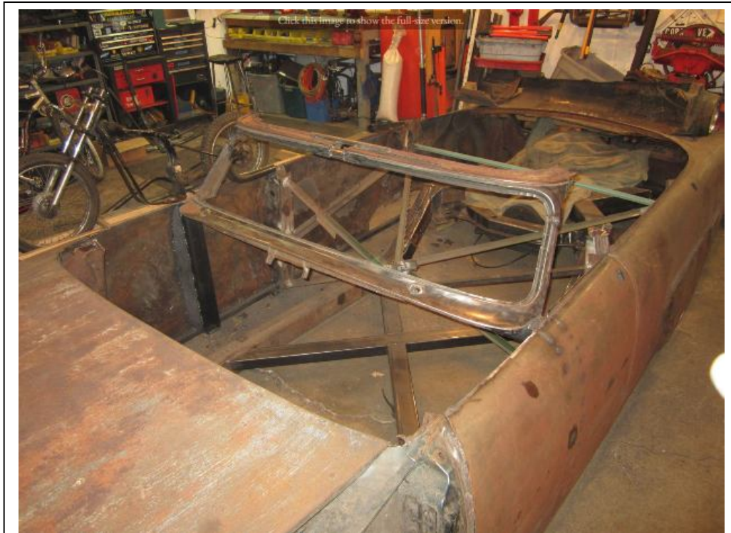
I cut the windshield frame loose and moved it back 18 inches and chopped 1/3 off the top.
