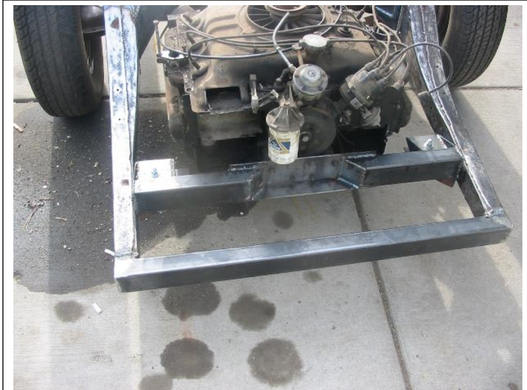
That second cross bar is a very burly engine mount. Rubber mounted with earl Ford F-1 mounts
