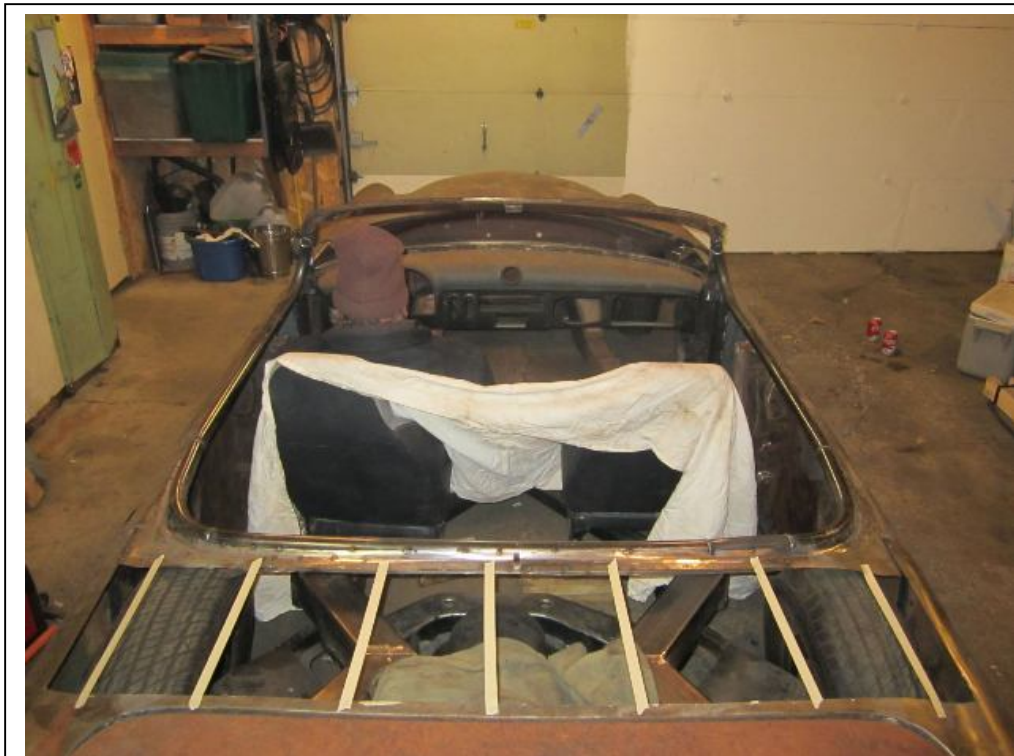
The rear deck was lengthened by a foot. There is some mock-up stuff happening in this picture.
