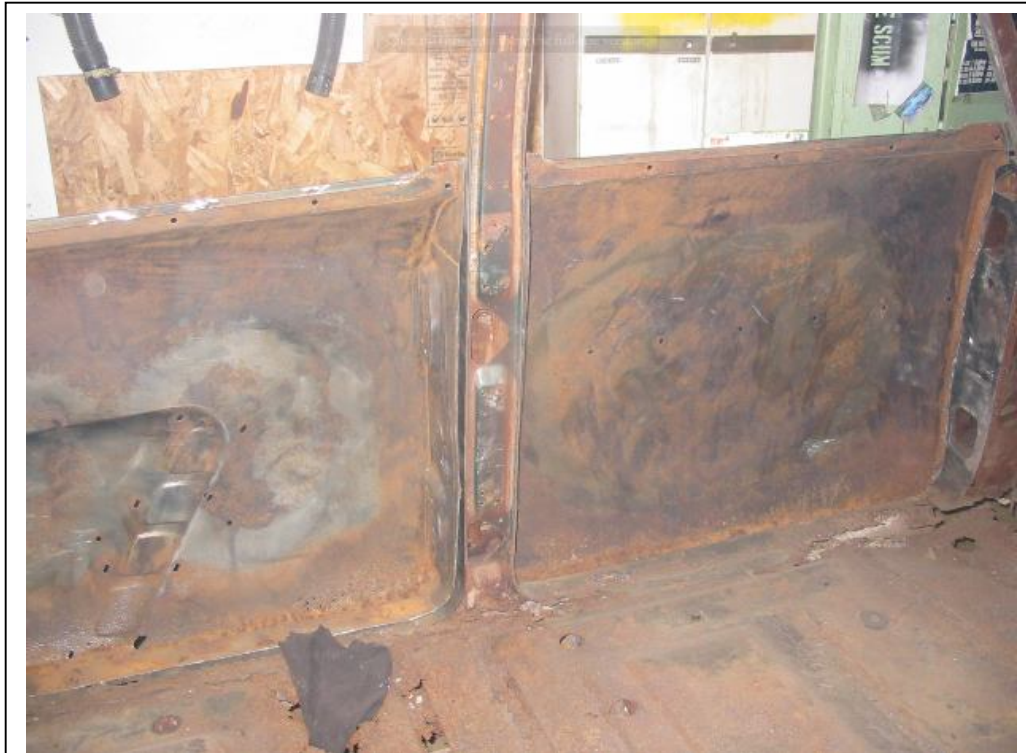
Here are the two driver doors skinned and welded in.
