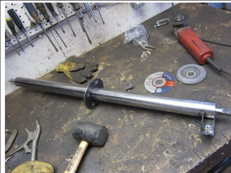
This is my intermediate steering shaft. I built it from scratch with some very primitive machining techniques. It is nearly 3 feet long and sits in the car totally horizontal.
