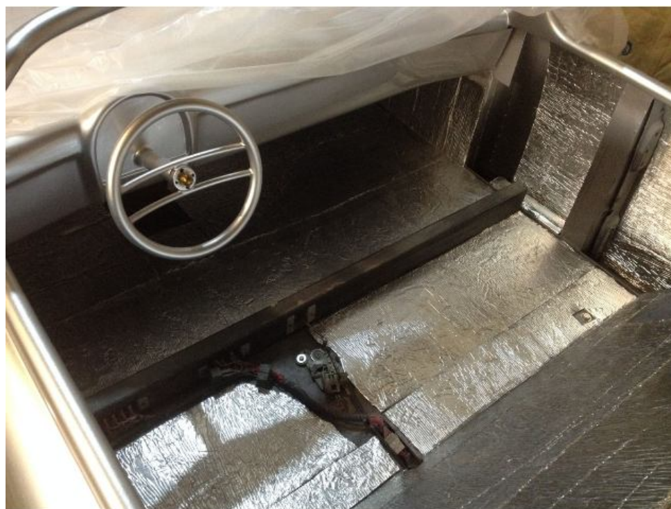
Poor man's Dynamat. Duct insulation.
