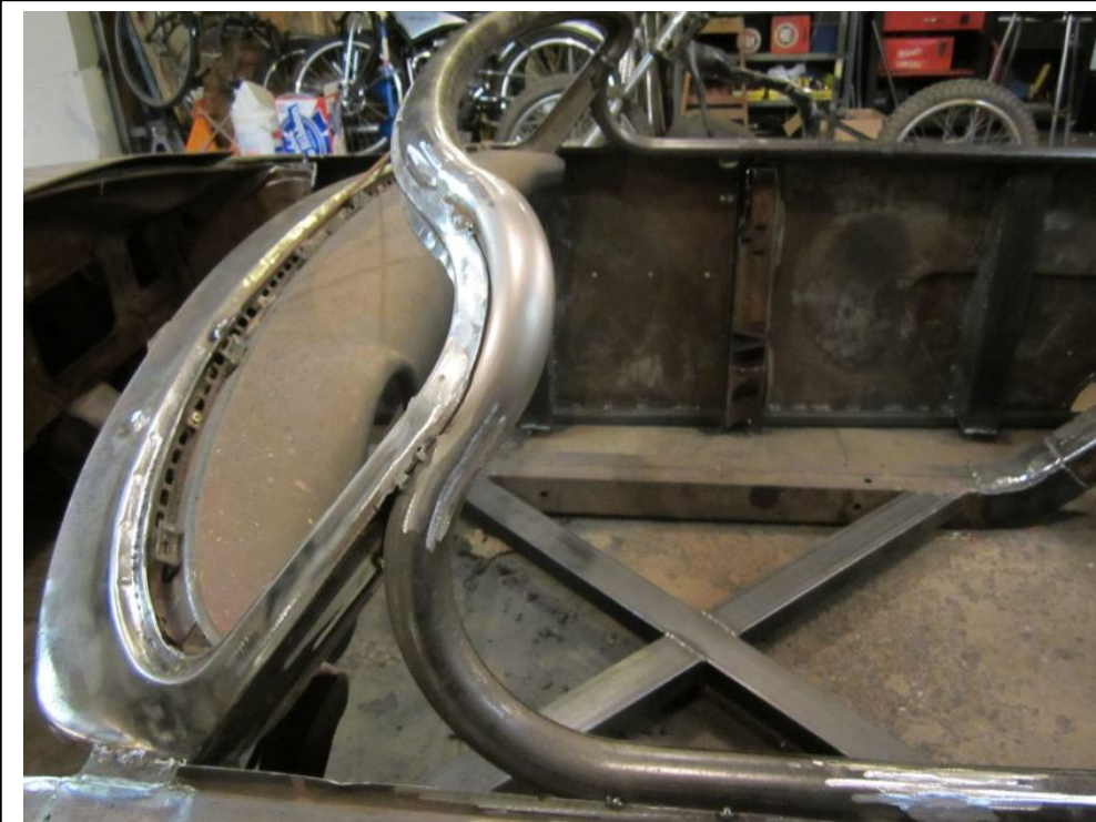
This is the perimeter tubing done. I had to use exhaust mandrel on the tightest bend.
