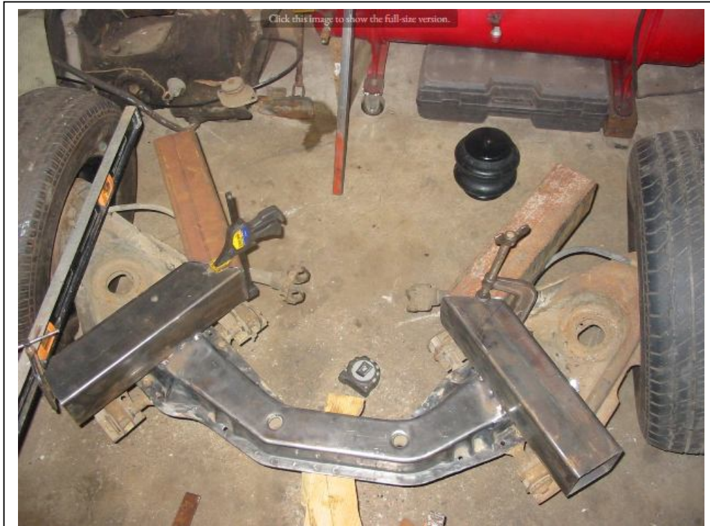
This is the Corvair rear subframe. I am adding 4x4 to it to graft it to my frame.
