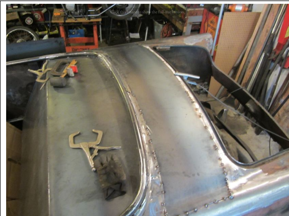
Filled the gap in my rear deck.
