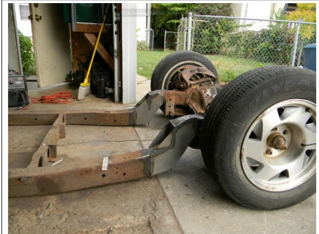
Sorry, the last one was out of order. September 2011 I welded on an S-10 subframe with a pretty healthy step-up.
