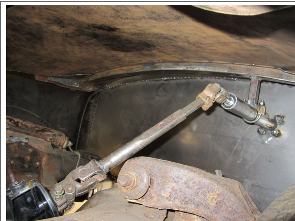
This is part of my steering; there are 3 sets of u-joints. It works surprisingly well. No slop.
