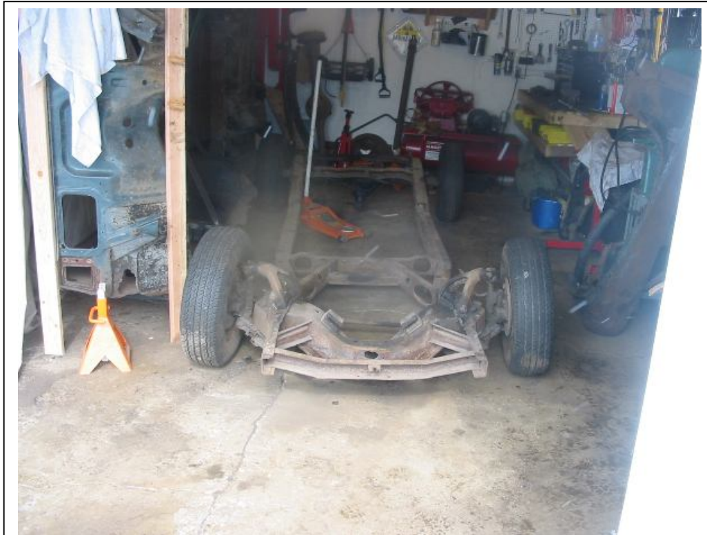
Pretty much everything got stripped off of the frame. In the end I used so little of it; I could have scrapped the whole chassis and been ahead.
