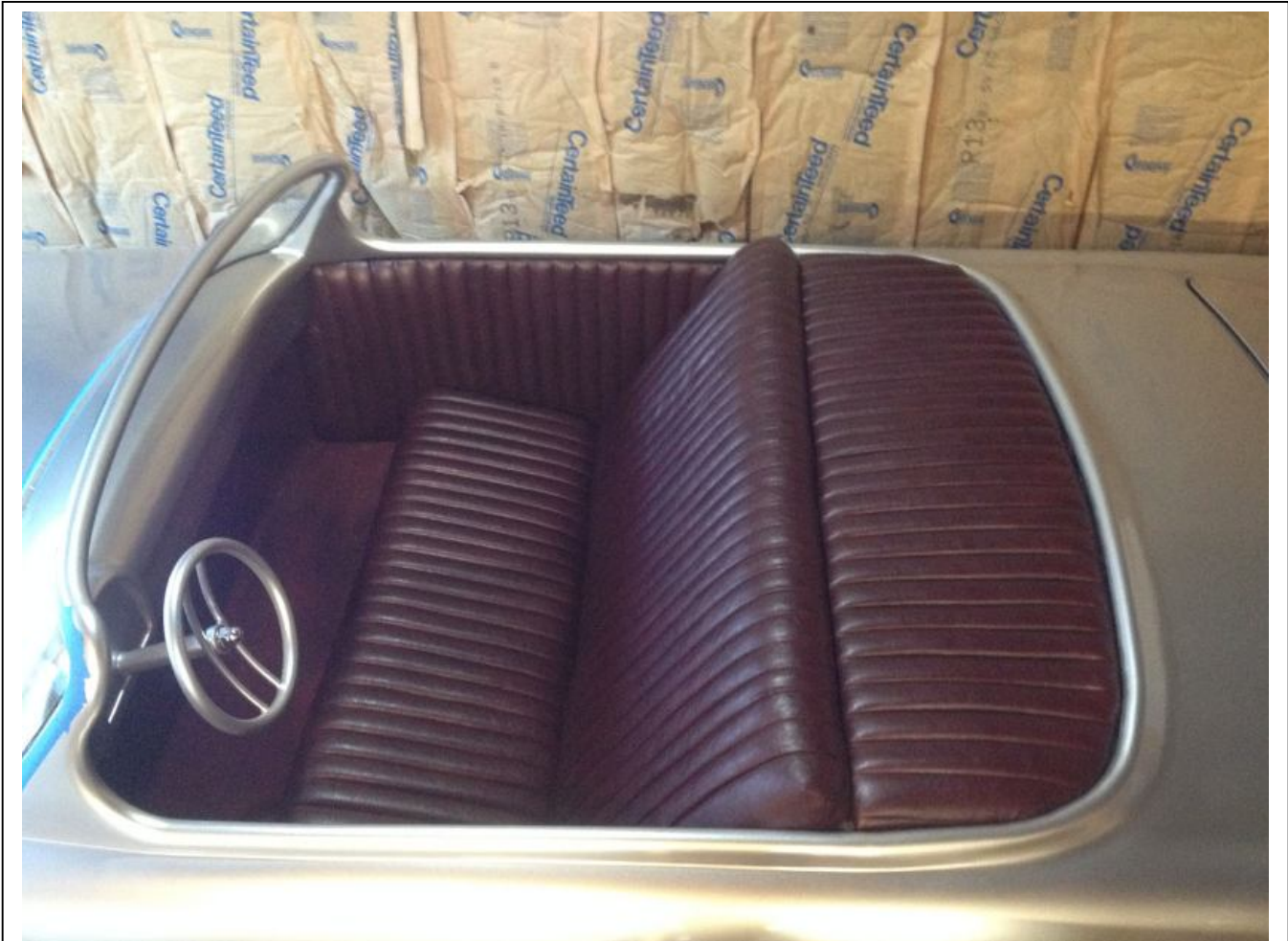
Oxblood tuck and roll. I had some good support and tutelage from Nate at Vinylux Upholstery.
