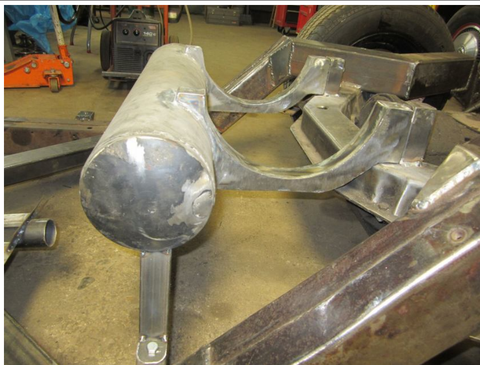
This is a three gallon air tank for the rear along with a cradle to mount my fuel tank.
