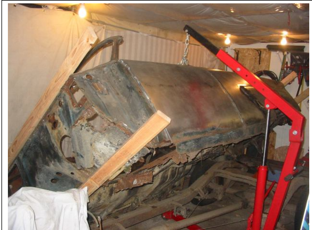
Tipping the body onto it's side.
