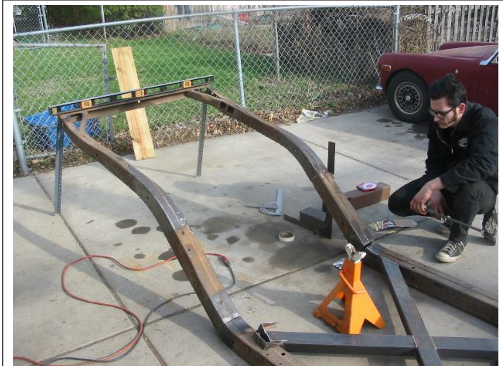
I pie cut the rear end of my frame to make it kick-up.
