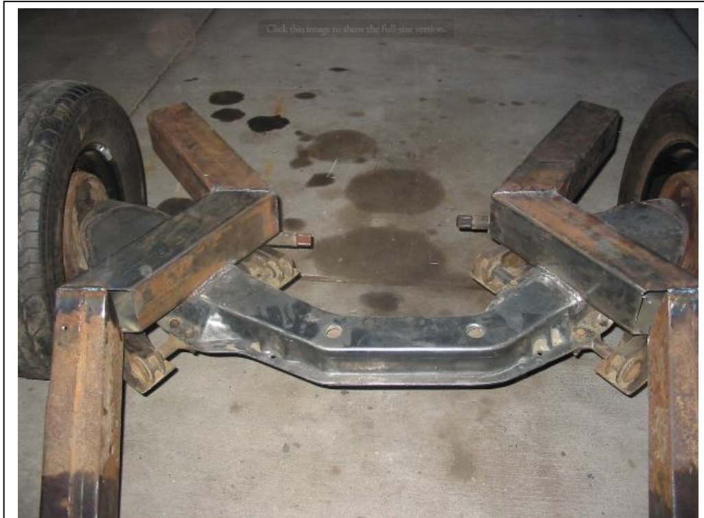
Here is the Corvair subframe connected to the rest of my frame.
