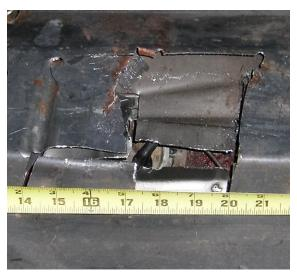
tested it successfully, and then reinstalled it – down in the hole I had made – and the installed test shows full tank @ full tank. We'll see how it tracks the rest of the way down! I'm pleased I could do it myself and keep the program on schedule. If ever you should be so inclined to search for that sender from 'Above' here's a photo of where to cut. The ruler shows the sending unit to be 17 inches from the right-hand (passenger's) wheel well,
