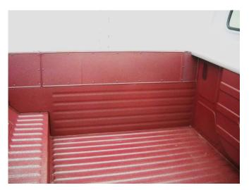
panel, so that the centerline of the first one is 5/8" in front of the original left panel. The remaining ones are spaced 7 3/4" on center, except for the one directly behind the cab. The center of it is 5/8" back from the cab. If you want to measure all from the front edge of the original panel the centers are: 5/8, 83/8, 161/8, 237/8, 315/8, 393/8, and 471/8. One angle is placed along the
