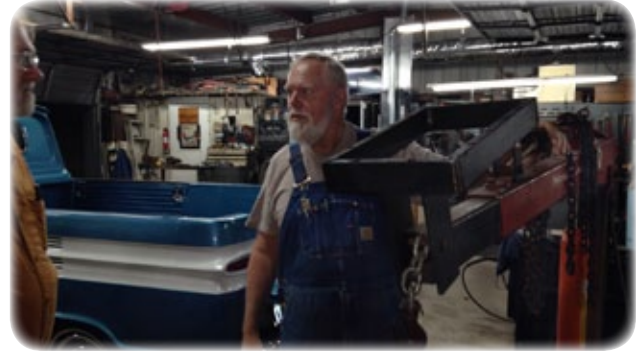
J.C. shows Larry the fixture he attached to his cherry picker hoist to allow him to change out an engine while the Corvair's on the lift.
