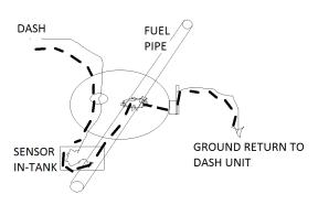
I've drawn those words that show the current flow from the dash unit into the tank and through the sensor, then up the pipe and out to the ground. That is what you must have.
