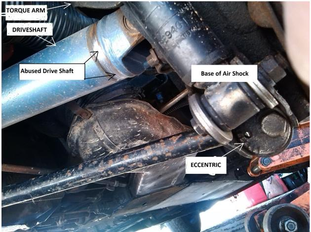
If you are working on your Late Model's suspension and forget to tighten the nut on your
