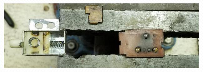
The switch is just a plastic slide piece in a housing (left) that holds a copper plate (top center) that makes contact with terminals on a circuit board (right) when you move it. I just cleaned and greased the slide, used a Scotchbrite pad to clean the copper plate and contacts and put it all back together. It worked great!
