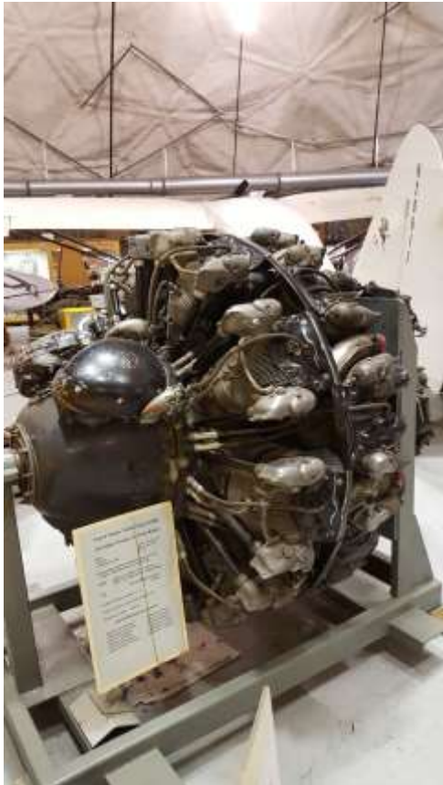
Pratt & Whitney R-2800 air-cooled radial engine. It powered such aircraft as the F6F Hellcat, the F4U Corsair, and the P-47 Thunderbolt. This one is on display at the Pioneer Aviation Museum in Fairbanks.
