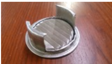
Top: Top of Vent Above: Bottom of vent before modification Below: Bottom of vent trimmed to fit drain holes
