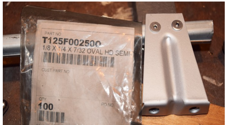
Figure 7. Attaching bottom mounting bracket with rivets and washers.
