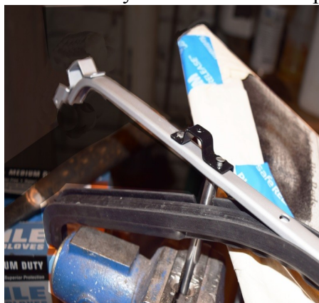
Figure 5. Reattaching window hinge rivets in the support frame.
