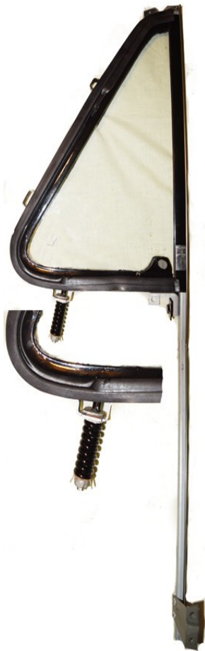
Figure 8. Completed vent assembly and close-up of tensioning
