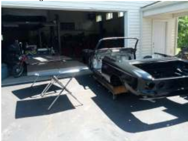
Got the featherfill surfacer sprayed. Now more sanding
