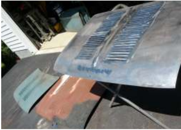
Everything but the doors are in epoxy primer. The doors are being shipped from California, none of mine were worth saving.
