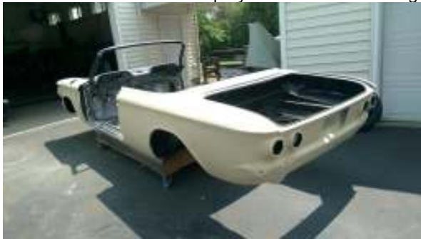
Got the featherfill surfacer sprayed. Now more sanding
