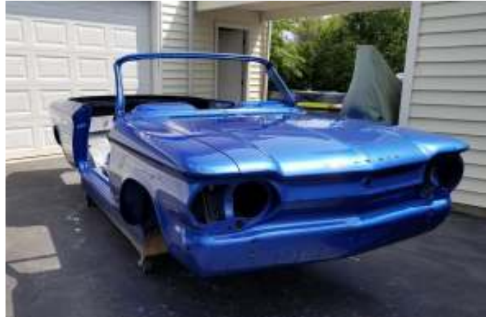
Everything but the doors are in epoxy primer. The doors are being shipped from California, none of mine were worth saving.
