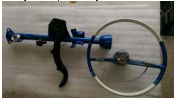
Steering wheel all painted along with column and ebrake:
