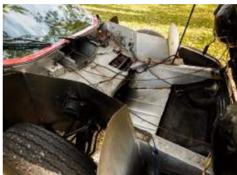
The “semi-monocoque” front of the car adds to chassis stiffness.
