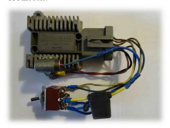
The module heat sink is about three inches square with about two inches more for the connector. The heat sink is about an inch or more tall.
