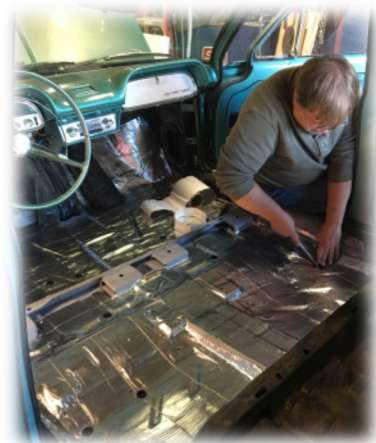
John Green installing sound deadening material on his new '61 Lakewood floor!
