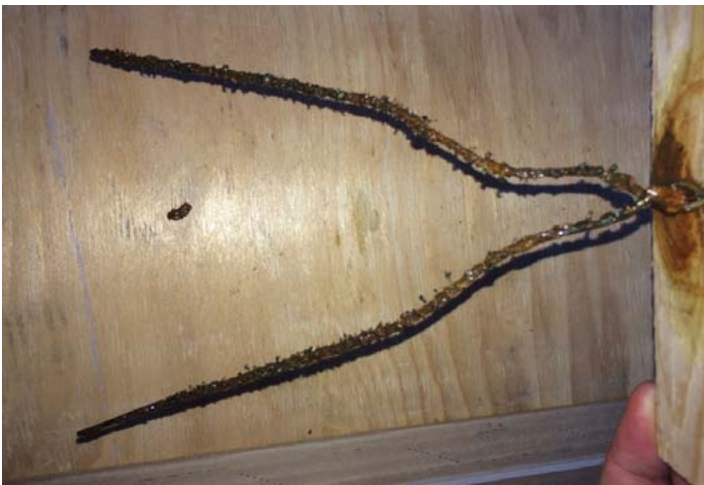
Anode with rust coating that is removed
