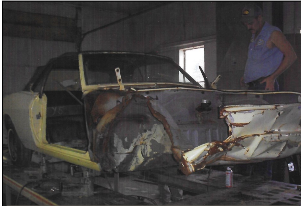
2007 - The car in Texas at the beginning of repairs, with the front right fender areas cut out.
