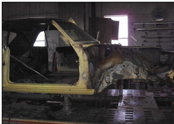
2007 - Up on the rack to straighten the frame and prep for the rebuild!
