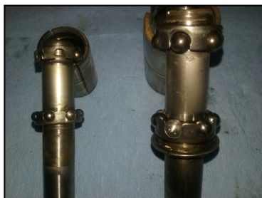
Fan Bearing assemblies for Early models, ('60-'64) (left) and Late models ('65-'69) (right).
