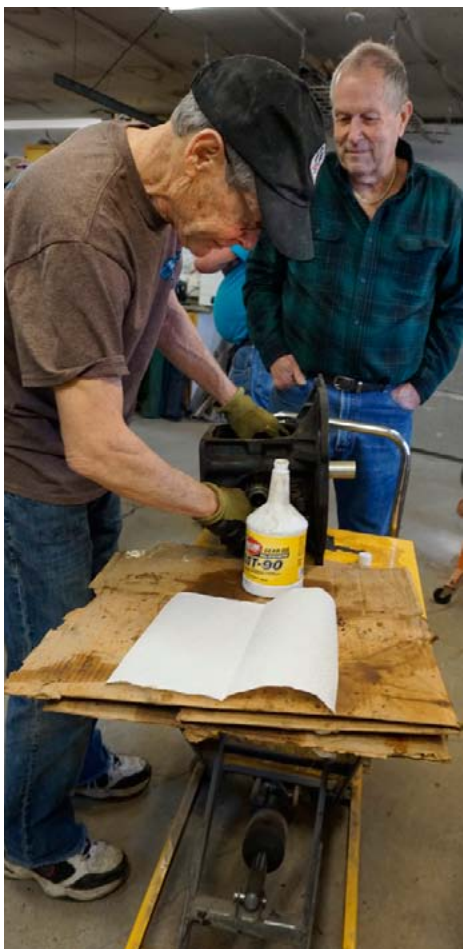
ABOVE: Scott Allison demonstrates the shrink tube method of PG cable repair on Ken Meyer's '66 500. Gary Jones assists.
