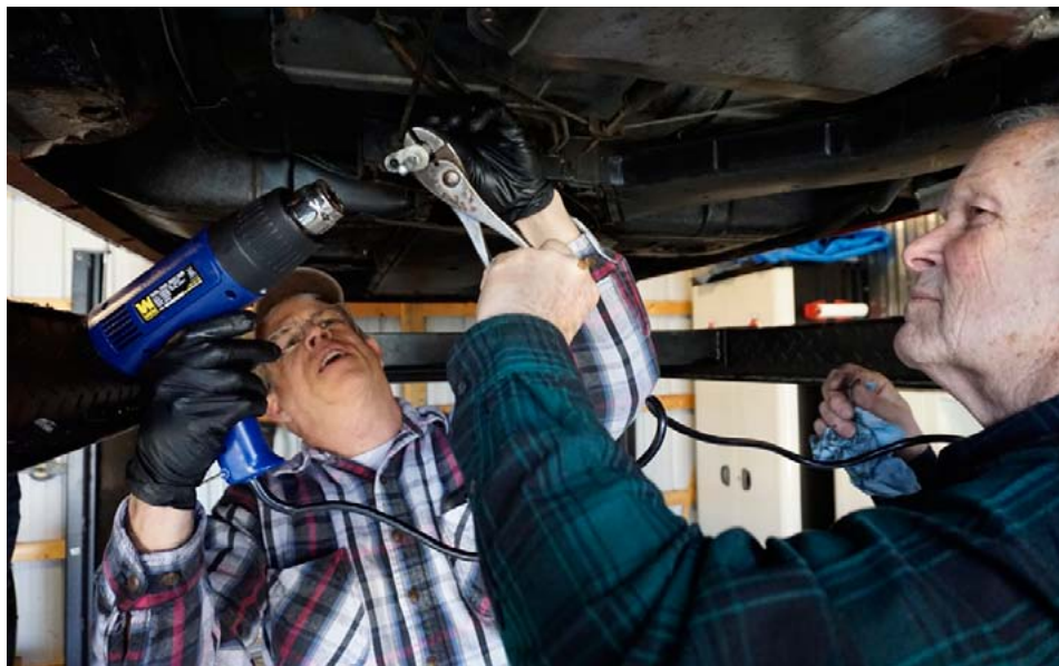
ABOVE: Scott Allison demonstrates the shrink tube method of PG cable repair on Ken Meyer's '66 500. Gary Jones assists.
