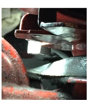
This view shows the cut-off bolt has almost enough clearance. When I added the nut I saw that I was clear but decided that the single thread sticking out was extra. Once the bolt is out of the nut it's not doing any good, so I snipped it just a little bit more and came up with this
