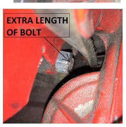
(on the left). Since this portion of the belt is always under tension, there would be no ballooning of the belt as the engine ran. So, I figured this was a good fix for my stripped thread on the GENerator of my 1961 FC.
