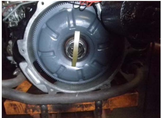
This shows a "tool" I made from an old diff sleeve and a piece of fiberglass to minimize wear on converter internals when running without a differential. I filled the sleeve with epoxy to seal it.
