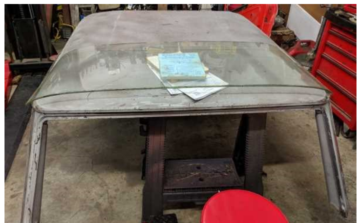
Donor roof and windshield standby for installation.
