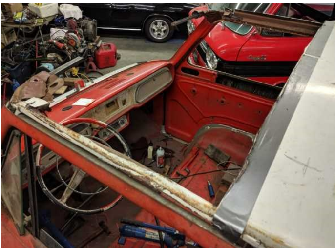
Drivers side top view of damaged roof skin and bracing cuts.
