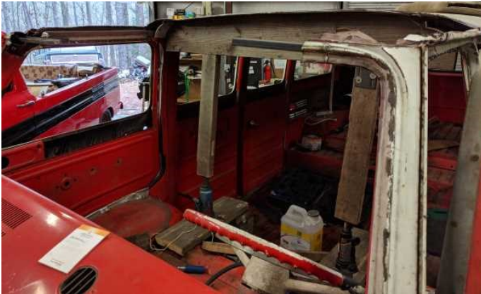
Drivers side front with alignment braces temporarily installed.
