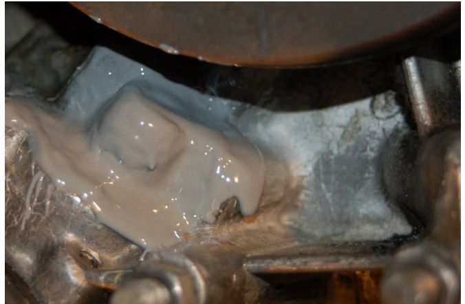
JB Weld applied over shaft bore.
