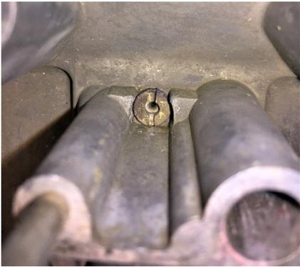
The tool has to be small enough to go straight down to the jet or you won't sit on the jet squarely – the tool MUST MATE with the Jet , like they say “nearly perfect”. It also has to be long enough to fit easily into the impactor that mounts on its top end.
