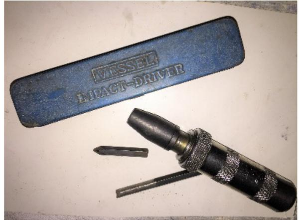
brass boys from way down in the hole. An IMPACT driver, that I have, uses a 5/16" hex drive. So I took a four inch piece of 5/16" hex and ground it round so it would fit down into that special area that hides the Main Metering Jet in our favorite carb.
