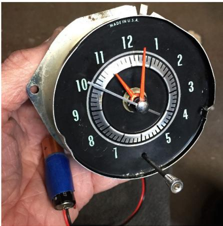
On the left is a view of the 'new design' (DC powered quartz clock with pulsing second hand) **including** the front-mounted adjuster stem – exactly at 6 o'clock. Ready to be reinstalled in any LATE or more realistically back on the dash of Fran's '64.
