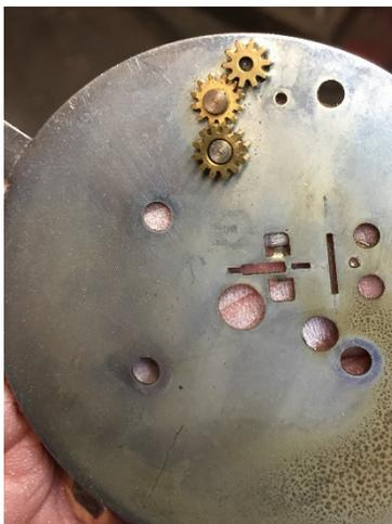
On the left you see the little guys that accomplish that 'turn around'. The long shaft, from the front, drives the top gear in the photo. Obviously turning all the others and carrying the 'turning' towards the center hole. The clock mechanism used to drive the hands through the center hole in this plate.
