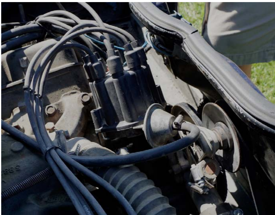
Spot the Corvair engine part on the '65 aluminum Oldsmobile engine in Nate McLanghin' LM Corvair. It serves the same function in the Corvair and Olds. Fanbelt idler .
