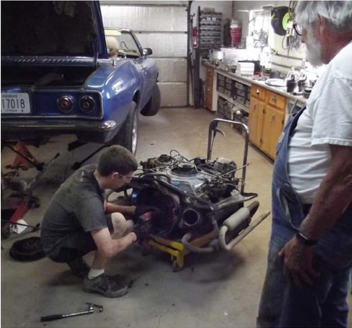
Larry Lee looks on as Alex Moats prepares to pull the bell housing on Larry's Corsa convertible. Alex replaced a damaged seal on the front main bearing.
