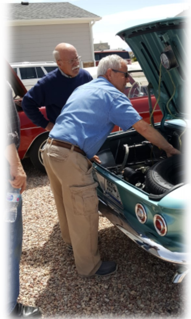
Ken works with Lynn to balance the carbs on his '64 Monza, using a two hose vacuum gauge.
