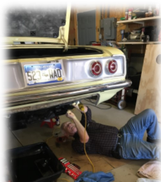
Pat picked up on the task quickly, removing the passenger side rockers, and replacing the lifters, one cylinder at a time.
