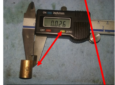
New bushing is considerably longer and thicker, better able to carry the load.
