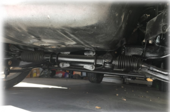
Rack and Pinion Steering added to the Corvair
