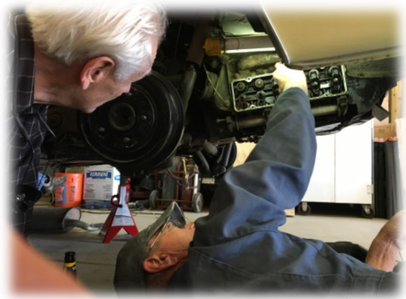
In preparation for replacing the lifters, Ray Schick (on the ground) provides a tutorial on how to remove the rocker arms, as Pat Carty looks on. Pat got his chance to turn a wrench on the other side of the engine.
