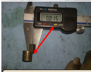
Note the length and thickness of the existing bushing.
