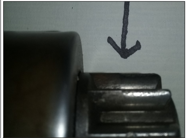
Note the significant amount of wear on the starter's gear teeth
