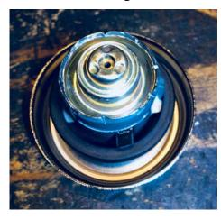
Finished fully vented cap with center section restaked.
