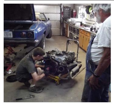
Larry Lee looks on as Alex Moats prepares to pull the bell housing on Larry's Corsa convertible. Alex replaced a damaged seal on the front main bearing.
