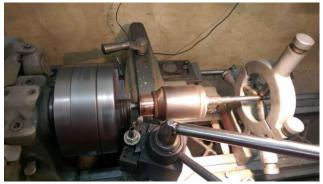
Armature turned down on lathe
