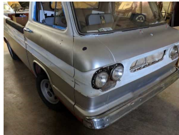
The gray base coat over the faded and prepped original red. Three coats with 24 hours cure between each.
