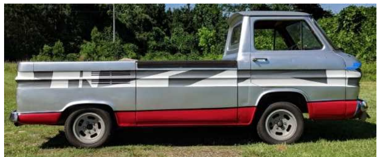
The white 'belly band' and red oxide 'water line' was masked and painted 3 coats. Dazzle camo applied one side at a time.
