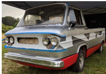
The white 'belly band' and red oxide 'water line' was masked and painted 3 coats. Dazzle camo applied one side at a time.
