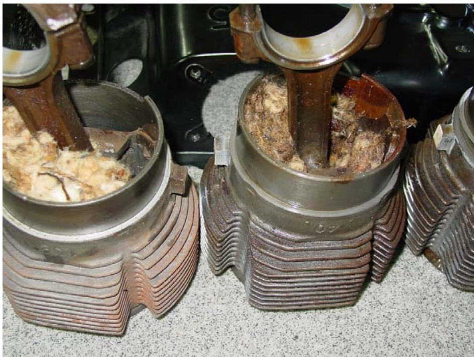
Sat for awhile after overhaul. Mike Dawson sent this photo of an engine he recently purchased. It had be overhauled, but sat for several years, long enough for the mice to set up a nice motel..
