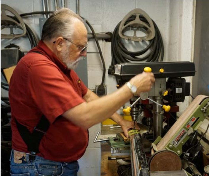
Ray Juenemann makes good use of the drill press in the Kalp Shop making holes for bumper guards.
