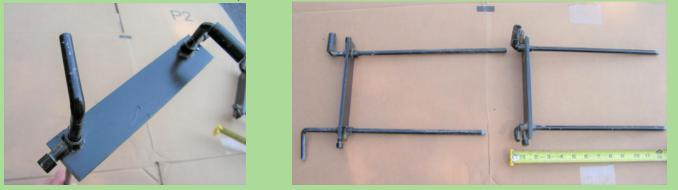
The rods are adjustable in and out through the steel plate, can be rotated, and can be locked with the thumbscrews on each one. One of the rods on each pair has an attached sleeve.
