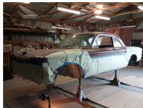
Masked and ready for spraying.
