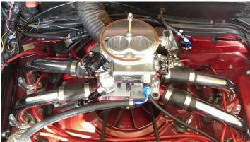
Back out of the garage. Travel maybe thirty feet and it dies. Tap the starter. Nothing. Crank the starter. Still nothing. Watch down the unit while cranking. One side is dumping gas like the pedal is stuck to the floor. Reset everything and reprogram it. No change. Still flooding. Quick call to supplier and they agree something is wrong. They send an entire new kit. After replacing every potentially bad part, the original kit is sent back.
