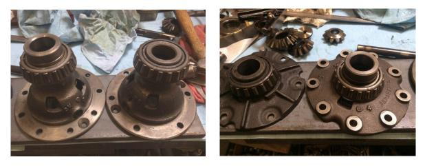
You can see the differences between the early and late differential components. The excess material above the bearings must be removed from the late parts so they'll fit in an early case.
