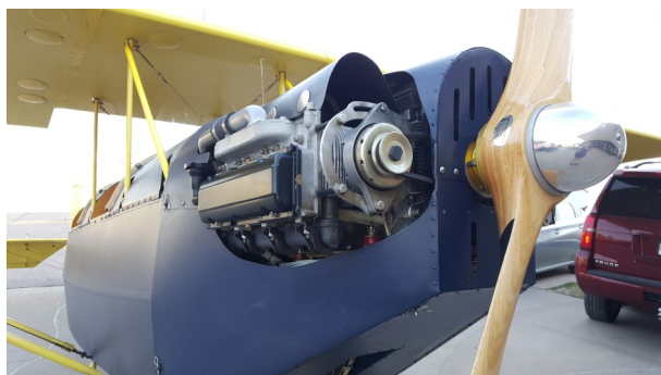
Modified Corvair engine is still recognizable, even without all of the sheet metal shrouding.
