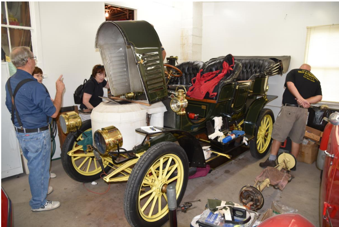
One of Charlie Johnson's personal Stanley Steamers. He drives it regularly on tours and parades. It requires refilling with water about every 50 miles and has a built-in pump so that you can get water from just about any convenient source such as from a river below a bridge. The large white mass under the hood is the boiler.
