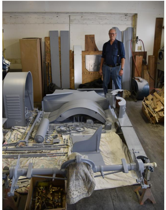
Chassis and body above, running gear, fenders and hood to right
