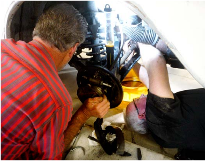
Alan Ballard (left) and Gary Israel are replacing a bad wheel bearing and axle on Gary's '64 Monza coupe.
