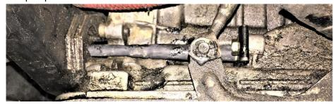
tunnel all the way up to the attaching screw at the PG. I went that far back to cover the possibility that the sheath may have been compromised, over the years, at that end. Now, everybody is covered...BIG time!
