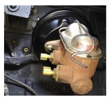
Then came the MC's time to be bolted up snug. Turns out I had to loosen up on those nuts when I mounted the steel lines as they are a nearly straight shot to the fittings on the firewall. I had to move the MC forward, so I could thread the lines back on, at the same time!
