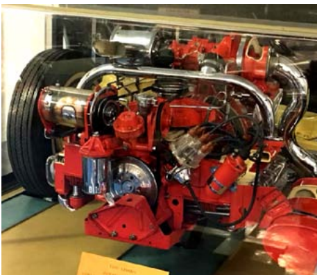
GM cut-away turbo drivetrain.
