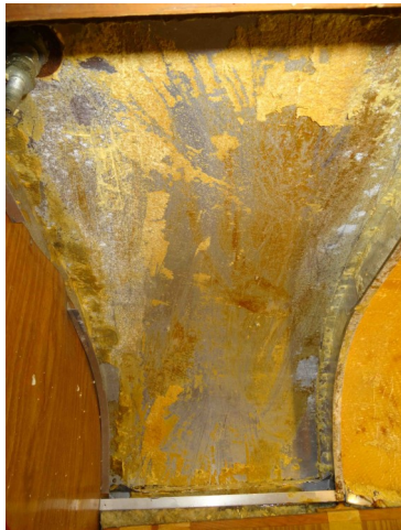
Passenger's side in front of the fiberglass corner with the foam gone
