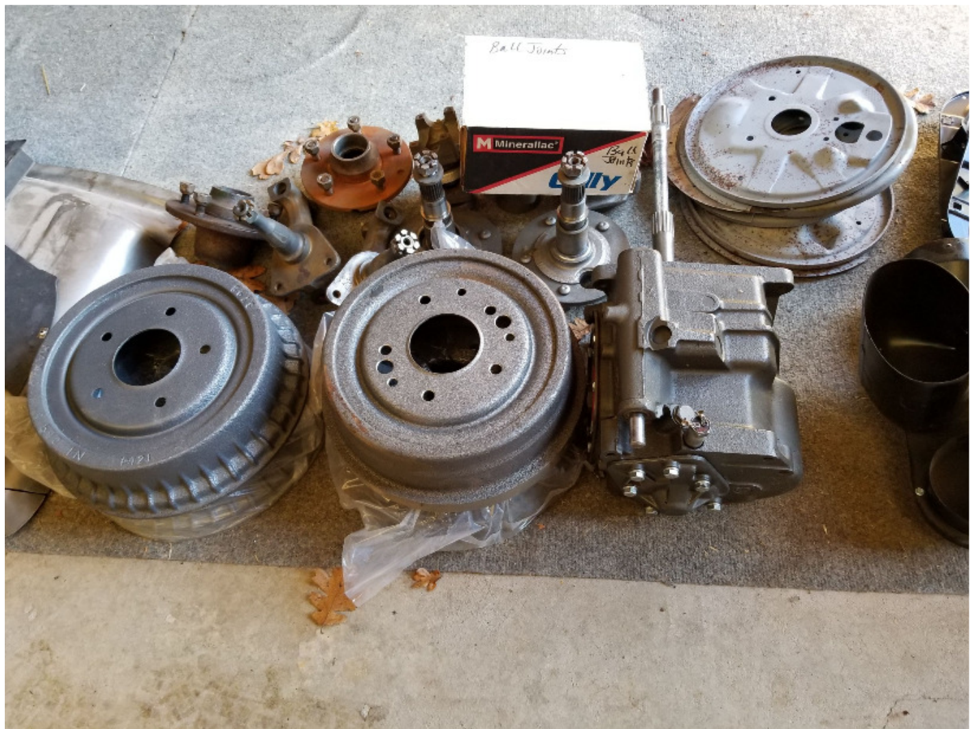
New brake drums and suspension parts, and a rebuilt four-speed transmission were included as well.
