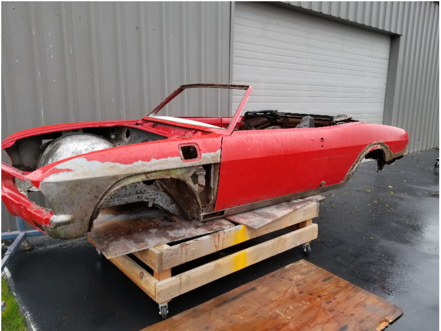
On the dolly at the body shop. The car is/was way too seriously rusted out for an actual restoration.
