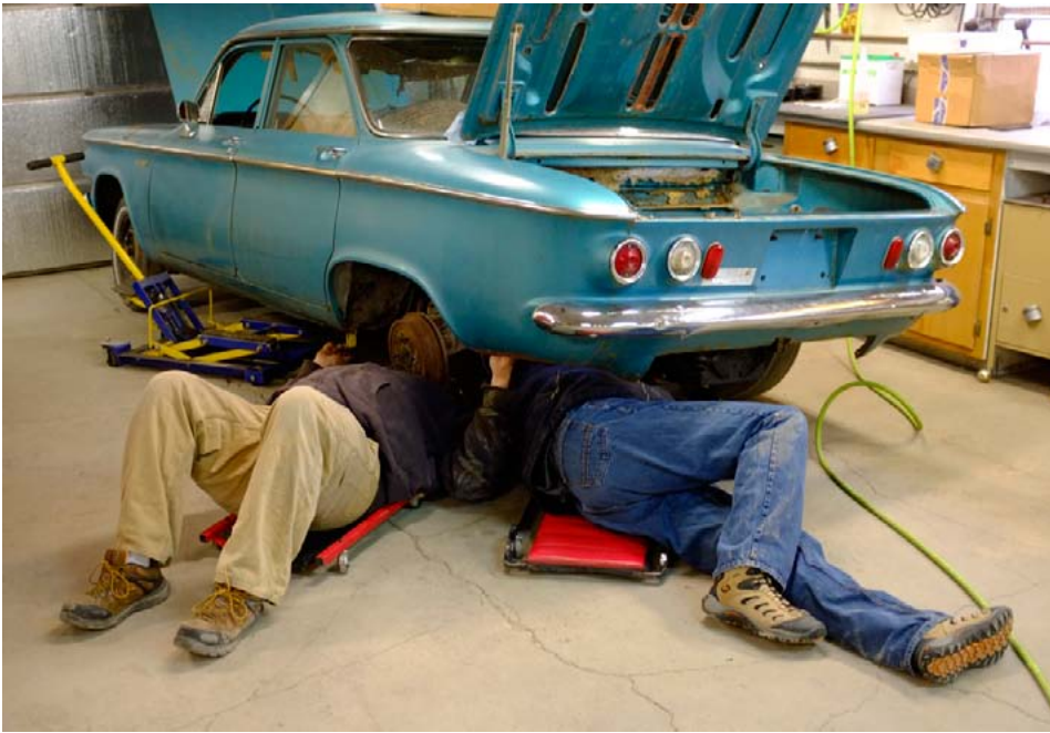
Tiffany Smith's '61 sedan didn't grow legs. Bill Smith and Greg Renfro were reinstalling the starter and checking wiring.
