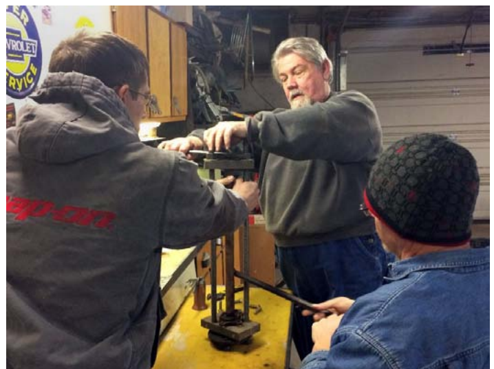
It was "all hands on deck" as Alex Moats, Terry Kalp and Mark Stever work to remove a rear wheel bearing from an EM axle. Mark Welte Photo.
